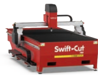
Pro 2500 (Pro 48) 2500mm x 1250mm cutting area (8' x 4')
